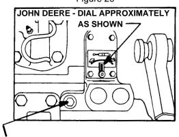
Typical plug for surplus relief flow line. Check carefully that it enters the reservoir before using. Note that the location varies with different tractor makes and models. A John Deere Tractor is shown.
